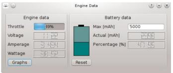
It monitors the amount of energy that came from the batteries and uses the batteries up to the point it is bingo time. Available battery packs allow the plane to yield up to 3 hours endurance.
